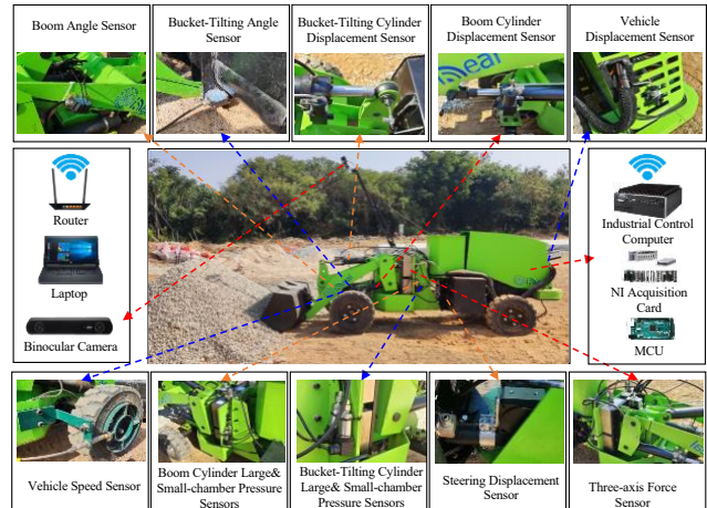
Fig. 17. On-site Layout of the Loader Excavation Trajectory Optimization Experiment
